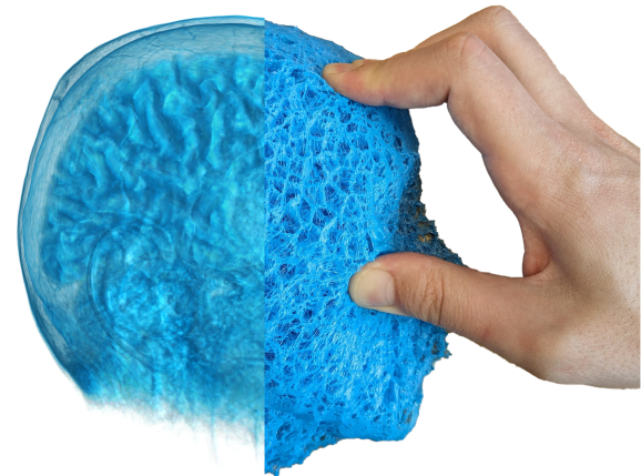
Fig. 4. A demonstration of the result (right) of the Squishicalization pipeline for a volumetric dataset of a human head (left), acquired by Magnetic Resonance Imaging (MRI). Local densities in the squishicalization correspond to scalar values within the volumetric dataset.
