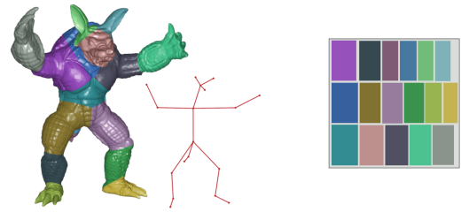
Figure 4: Visualization of mesh segmentation driven by the skeleton (left) and texture layout with regions assigned for each sub-mesh (right).
