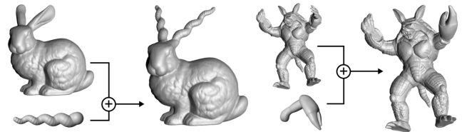
Figure 18: Transfer of surface regions of two models. The bunny's ears are replaced by horns (left), the armadillo's front paw is replaced by a pincer (right).
