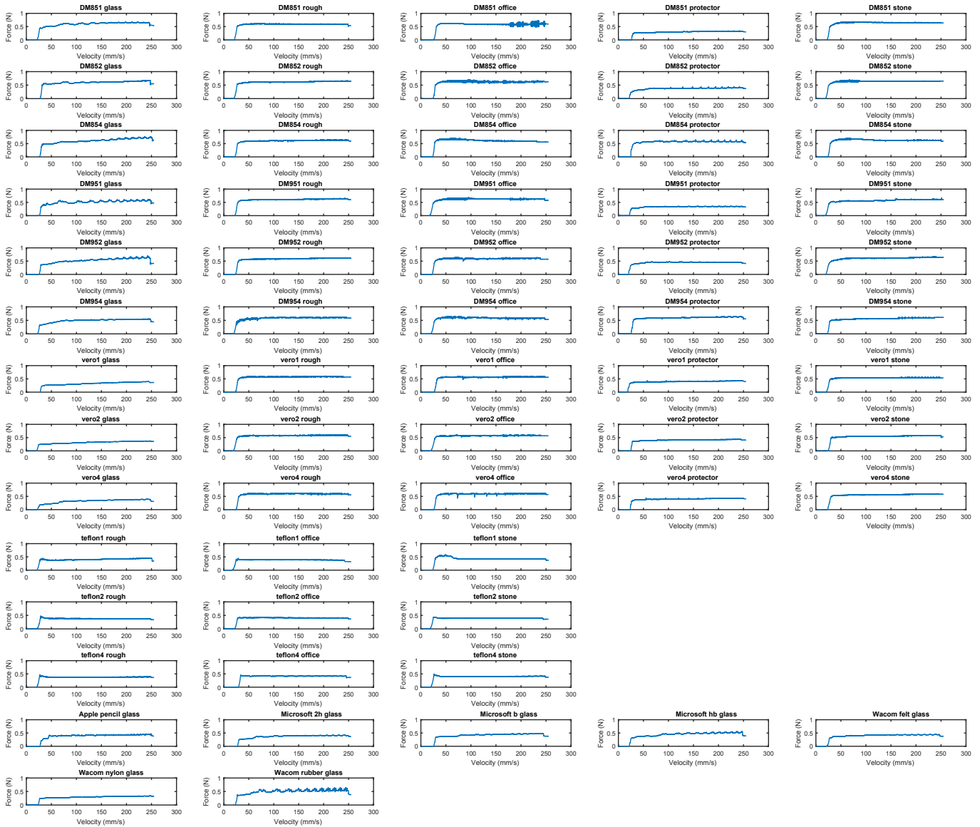
Fig. 7. Friction measurement of 3D printed and commercial styli recorded using our setup.
