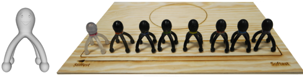
Figure 14: Left: a rendering of the original octopus model. Right: all printed octopuses ordered by stiffness.
